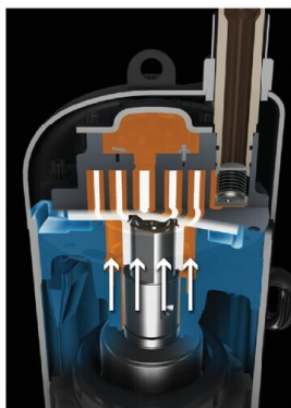
The force pressing the movable scroll decreases during low-load operation.
